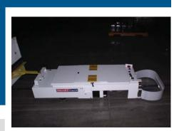
No. of AGCs: Operational: August 2006 System Type: Parts Delivery Guide Path: Magnetic Tape System Active: 8 hours per day, 5 days per week
