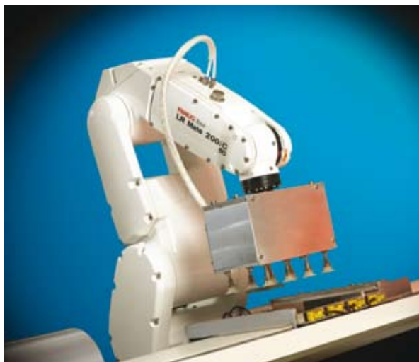
Cleanroom LR Mate 200iC/5C - the right choice for semiconductors & pharmaceutical applications!
